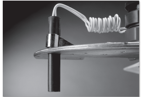
Figure 10. Heater installed on an S70 switch plate.
